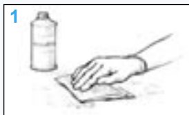
Figure 6 Clean the surface. Use a solvent, if necessary, to remove all contaminants.
