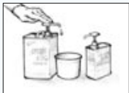
Figure 2 Dispense the correct proportions of resin and hardener.
