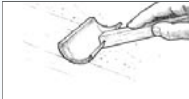
Figure 31 Tip off the coating by dragging a foam roller brush lightly over the fresh epoxy.
