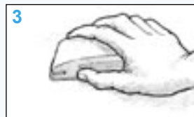
Figure 8 Sand non-porous surfaces. Provide a texture for the epoxy to key into.
