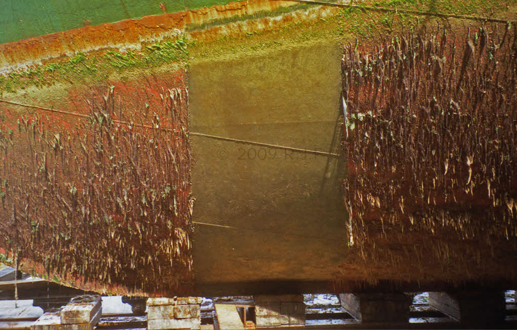
This picture shows a trial patch of Copperplus that was applied to a tug that was moored in Fowey harbour for two years. When slipped the Copperplus was virtually clean while the remainder of the vessel has a thick covering of growth of all types. The remainder of the vessel has been coated with a well known brand of commercial antifouling.
