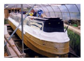
The illustration shows a vessel which has been grit blasted and masked up ready for the application of Hempadur 45140. Hempadur 45140 is a high performance priming system which will provide a priming or finish coat. It can overcoated with Polygloss or a conventional single pack finish.
