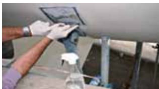
Wet scrape to remove old antifouling
