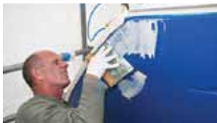
Fairing any defects
