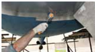
Apply Gel Protect with roller
