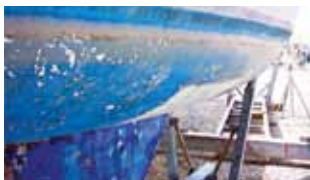
Paint blisters and lifts
